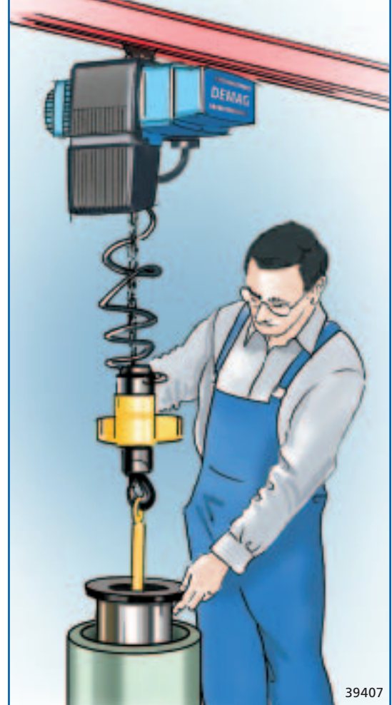
Smooth and precise positioning of a coil in a decoiler
